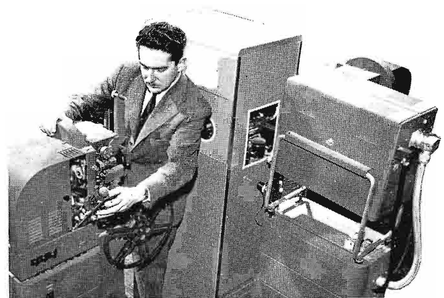
FIG. 6. Jules Maleone, RCA Service Company Engineer, is shown inspecting WEAU's two TP-16F projectors and TK-20D Film Camera, along with the Super Projectall. All of these units have worked out well in WEAU-TV's operation.
