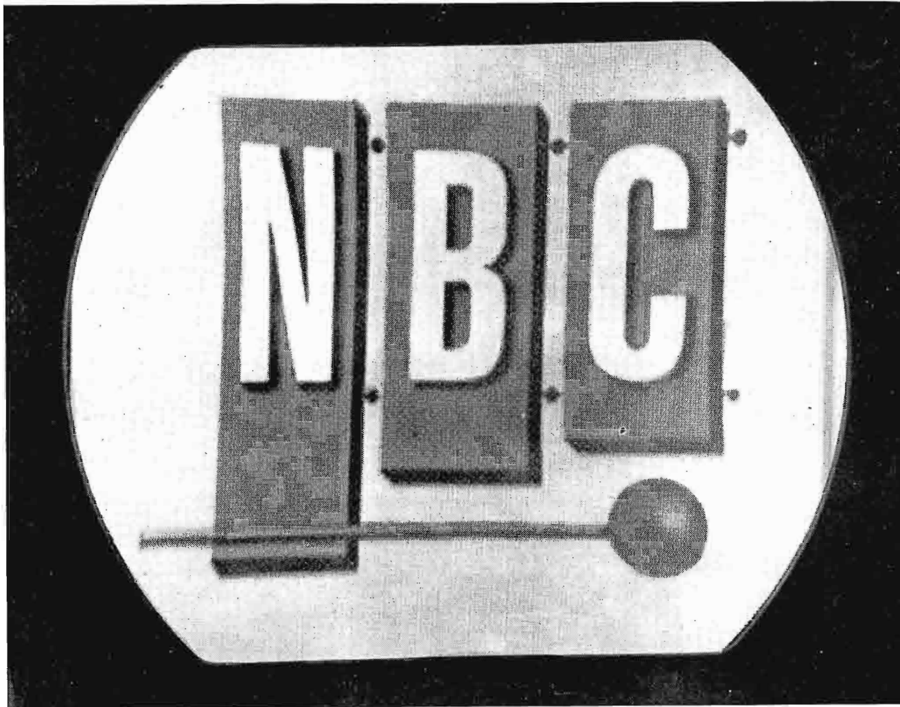
FIG. 2. Station test pattern revealing how WA-8A Color Stripe Generator enables any TV station which is equipped to transmit network color to add a narrow color stripe to its regular black and white television signal. On color home receiver tube a thin vertical stripe of greenish yellow color appears at the right hand edge of the picture as shown above.
